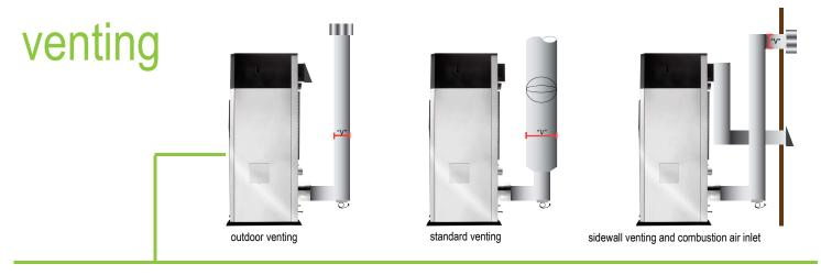
For ease of installation, the fully condensing Dynaforce can be vented individually in a Category IV positive pressure venting arrangement or they can be vented in a common chimney resulting in a Category II venting system.
